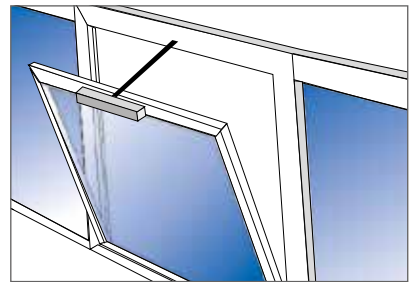
Bottom-hung window, inward opening at the top, with chain drive
