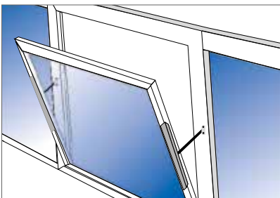
Bottom-hung window, inward opening at the top, with drawbridge chain drives
