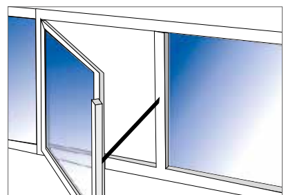
Side-hung window, inward opening, with chain drive
